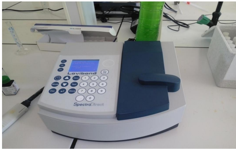
Figure 9: Spectrodirect de type Lovibond (photo personnelle)
