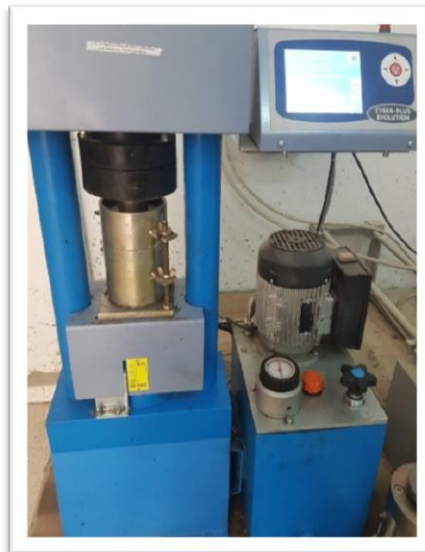
Figure 2.16: La presse de compactage
