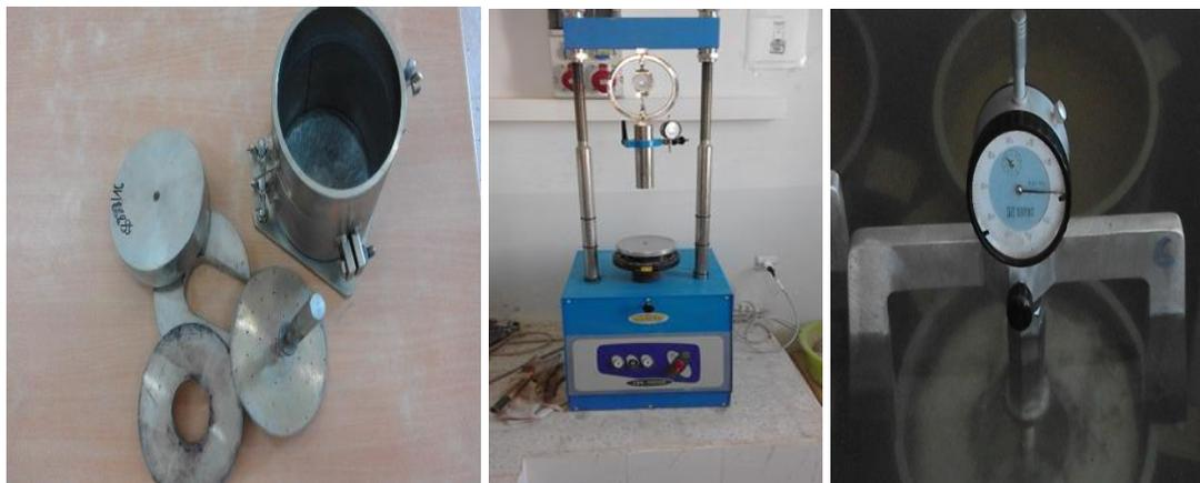
Figure III.21 : Appareillage – essai CBR.
