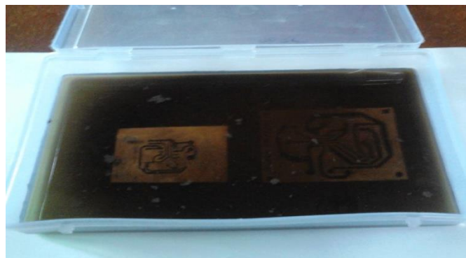
Figure3.11 Etching step for removing unwanted copper from PCB
