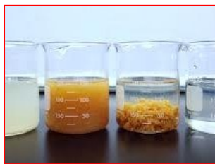
figure II-1 treatment water by coagulation and flocculation
