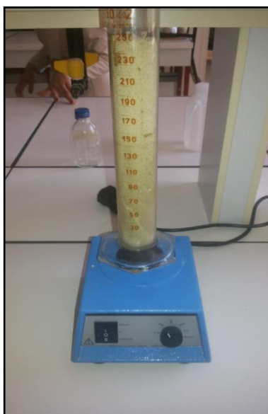
Figure 7: Test de tassement.
