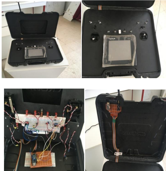
Figure 3. 12. Radio controller based on arduino and nRF24I01
