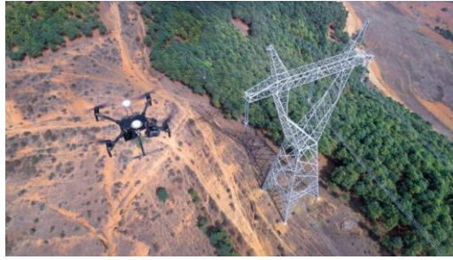
Figure 1. 21. Quad-copter used for power line inspection monitoring
