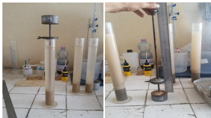
Figure III.8 : Essai Equivalent de sable
