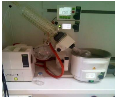
Evaporation du solvant
