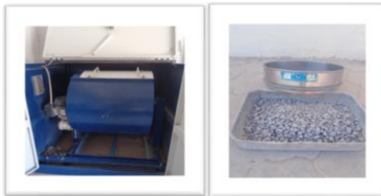
Figure III.6. Essais de Los Angeles
