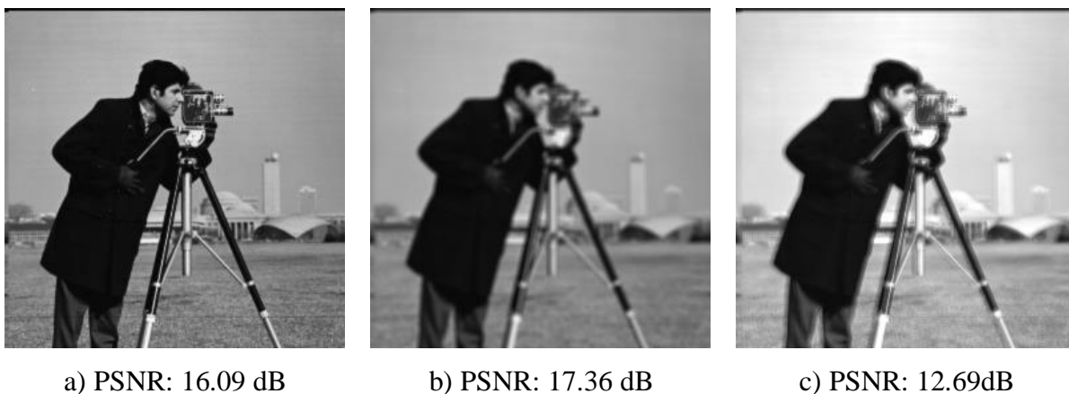
Figure 3.25: Hardware Gaussian blur with 5x5 kernel and a) \sigma=0.5 b) \sigma=2 c) \sigma=8
