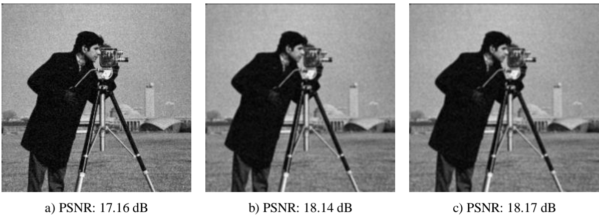
Figure 3.22: Hardware Filtered image with 3x3 kernel and a) \sigma=0.5 b) \sigma=2 c) \sigma=8
