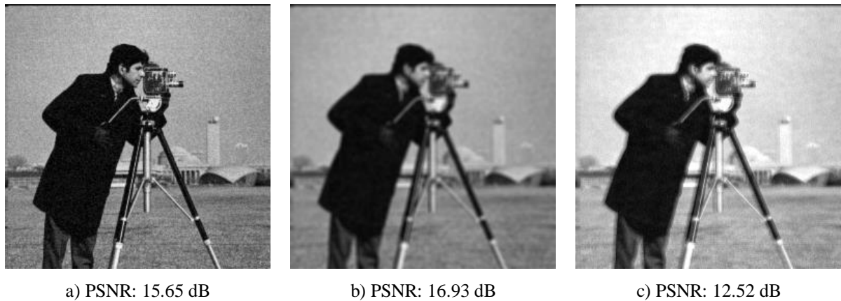
Figure 3.23: Hardware Filtered image with 5x5 kernel and a) \sigma=0.5 b) \sigma=2 c) \sigma=8
