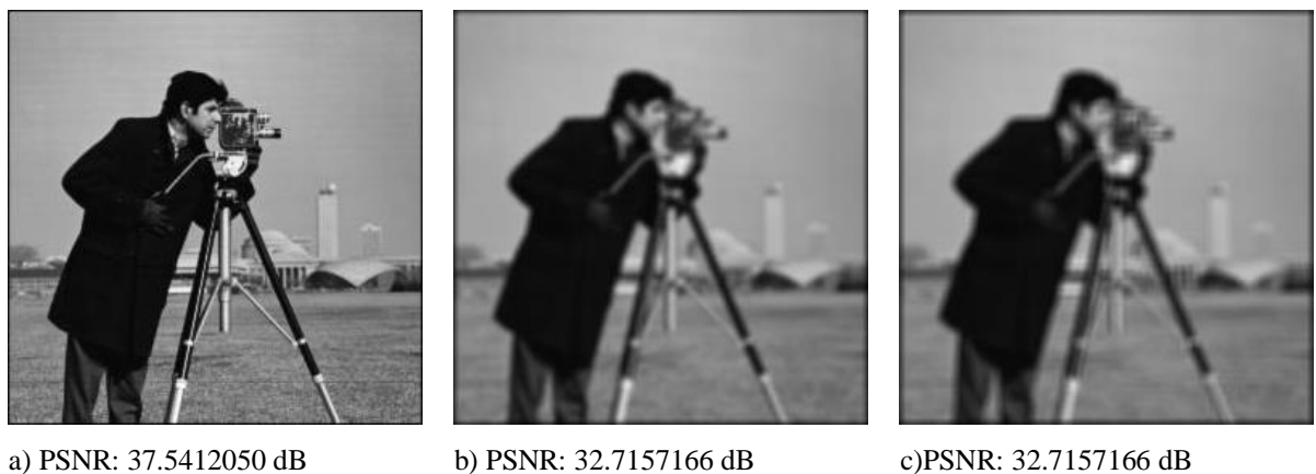
Figure 1.14: Gaussian blur with 5x5 kernel and a) \sigma=0.5 b) \sigma=2 c) \sigma=8
