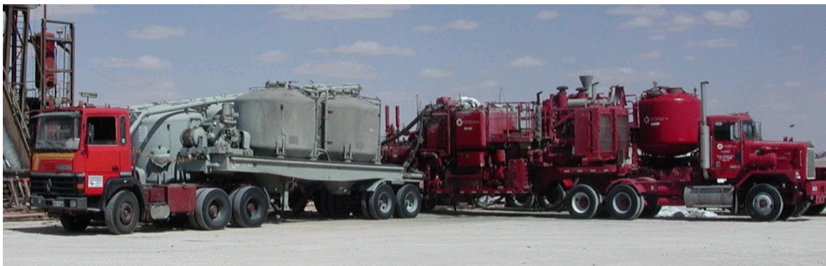
Figure I.14: Unité de Cimentation [4]
