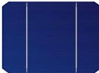
Figure. I. 9: Plaque de silicium monocristallin.
