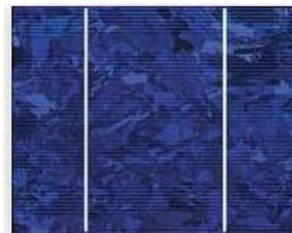
Figure. I. 10: Plaque de silicium poly-cristalline.
