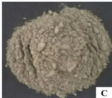
**Figure 2.1.** Echantillon de ciment CEM I (CPA 42.5 R).
