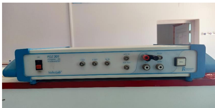
Figure II.11. Potentiostat VoltaLab 40 (PGZ301).
