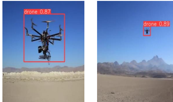
Figure 3.26: Drone detection using YOLOv8.
