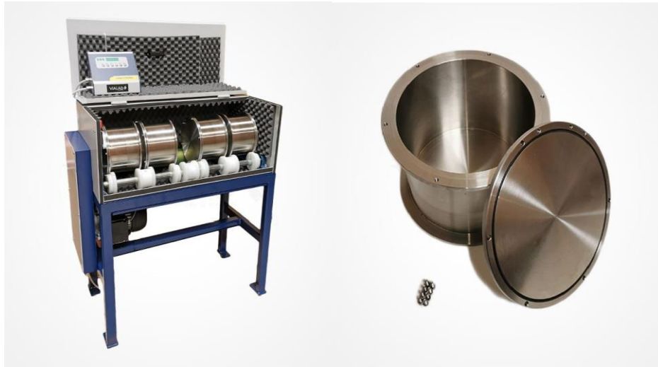
Figure III. 5: Appareillage Micro Deval
