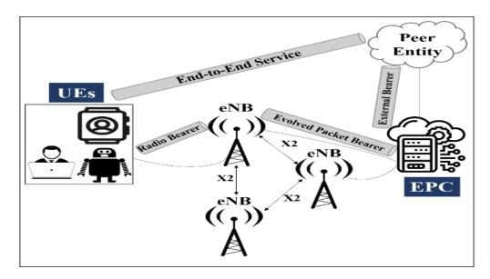
Figure 2.10 End-to-End QoS scheme in 4G LTE network.
