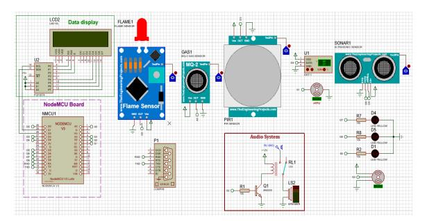
Figure 4.13 Circuit diagram of the smart environment system simulated using Proteus.
