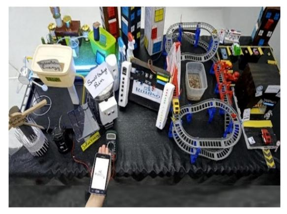
Figure 5.40 Top view of the extended IoT/M2M smart building to smart city prototype.
