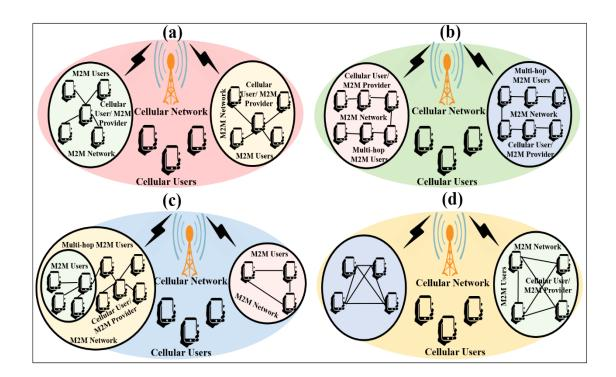
Figure 3.12 Converged mobile networks, including WSNs, MCNs, and M2M networks.
