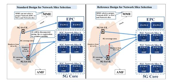
Figure 3.7 Standard and Reference Designs for Network Slice Selection.
