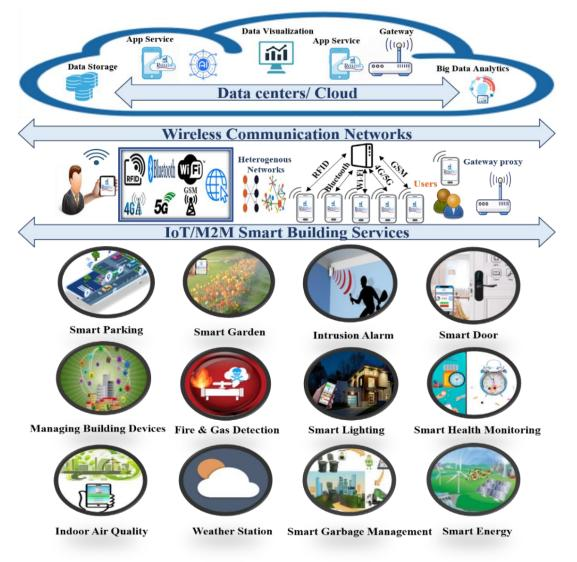
Figure 5.1 IoT/M2M smart building architecture.
