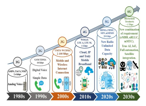
Figure 2.8 Existing and expected mobile cellular networks evolution till 2030.
