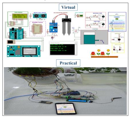
Figure 5.7 Illustration of the garden irrigation automation system.
