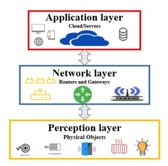
Figure 2.2 Three-Layer IoT Architecture.
