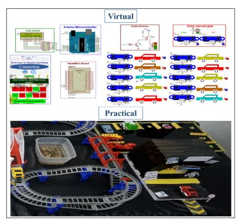
Figure 5.4 The proposed system prototype for smart parking.
