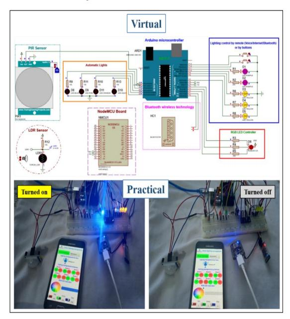
Figure 5.21 Smart lighting management by Remote (Voice/Internet/Bluetooth) or by Push Button Switches.
