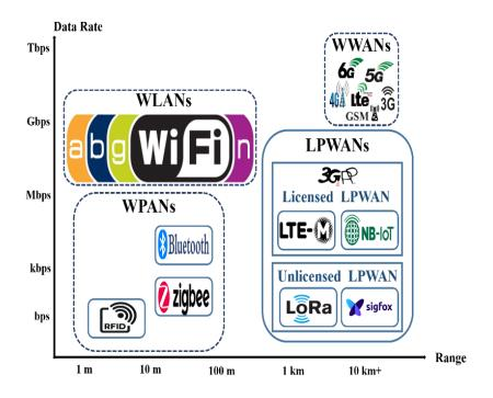
Figure 2.7 IoT/M2M communication technologies.
