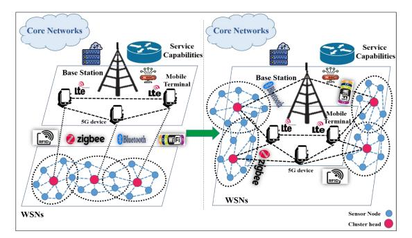
Figure 3.9 Converged network architecture for WSNs and MCNs.
