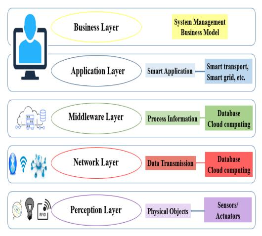
Figure 2.3 Five-Layer IoT Architecture.
