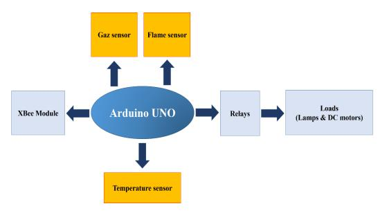
Figure 4.3 The block diagram of the master control board system.
