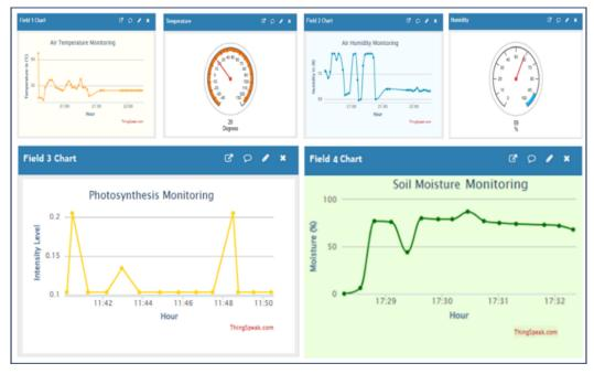
Figure 5.9 Garden Irrigation Monitoring System on ThingSpeak.
