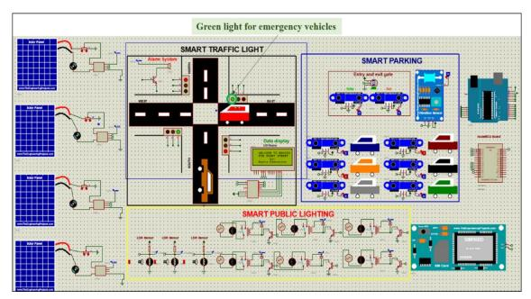
Figure 4.22 Schematic of the smart street system simulated using Proteus.
