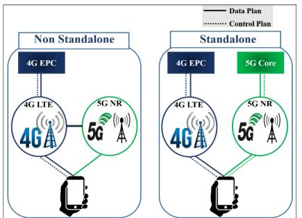
Figure 3.2 Non-Standalone and standalone deployment.
