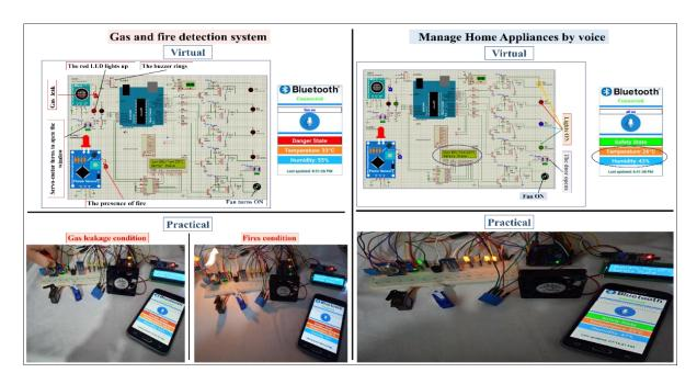
Figure 4.11 Implementation of M2M smart home automation.
