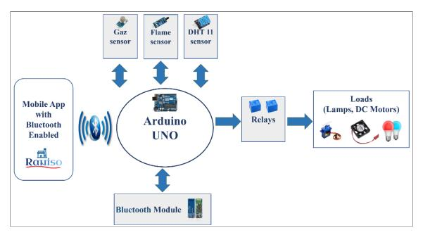
Figure 4.8 Block diagram of the system architecture.
