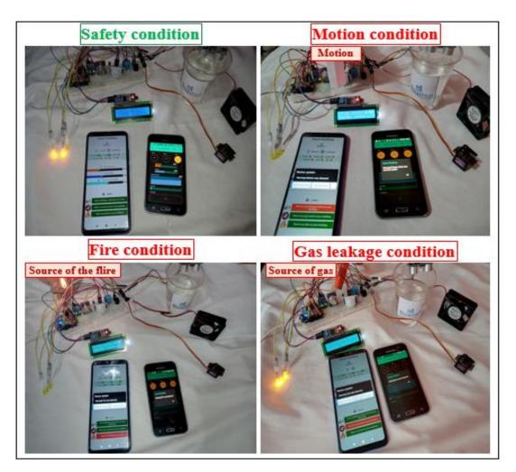
Figure 4.17 The proposed IoT/M2M smart environment system in different conditions.
