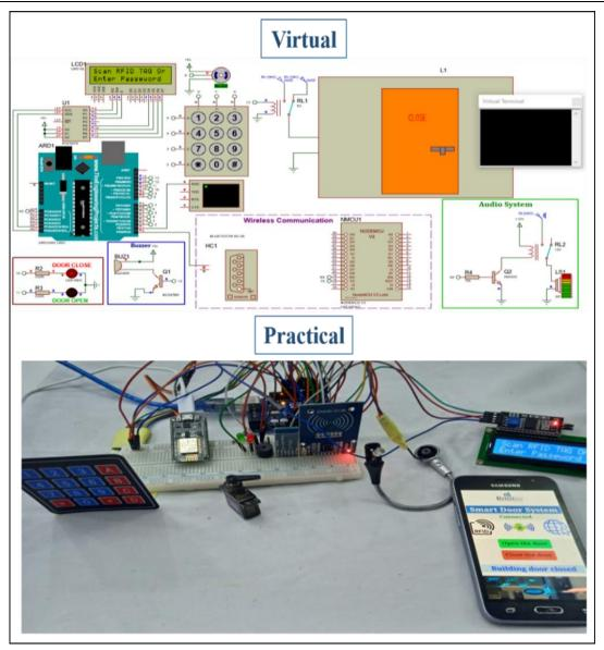
Figure 5.13 Prototype of a smart door system.
