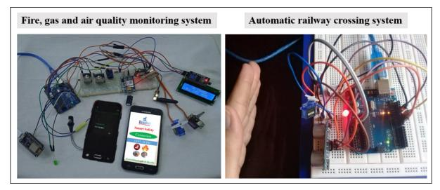
Figure 4.21 The implemented smart safety system.
