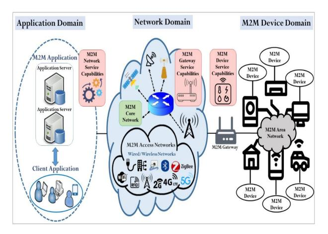
Figure 2.5 The architecture of M2M communication.
