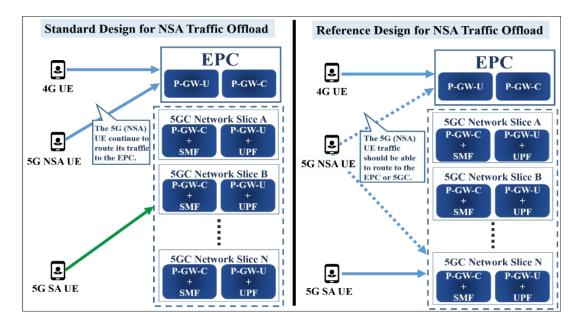
Figure 3.8 5G NSA UE Traffic Offloading.
