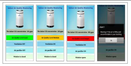
Figure 5.28 Indoor air quality monitoring interface on the Raniso.
