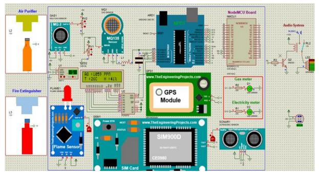
Figure 4.20 Schematic of the smart safety system simulated using Proteus.
