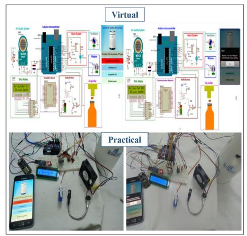
Figure 5.27 Indoor air quality monitoring system.
