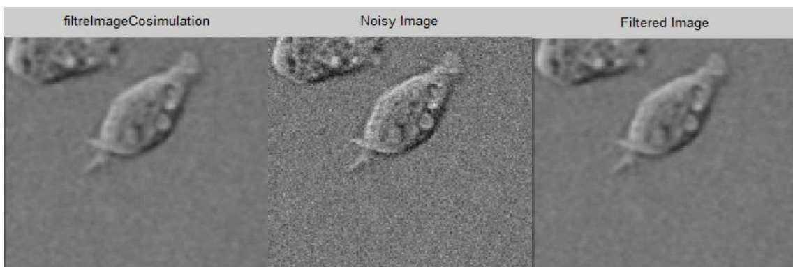
Figure II. 19 Hardware -Simulation filtered image with 5x5 kernel and variance noise=0.003
