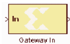
Figure II. 5. Gateway In block
