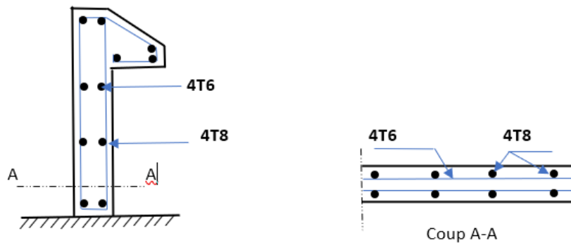
Figure IV.3 Reinforcement scheme of parapet
