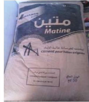
Figure III-4: Ciment CEM II B 42,5.
