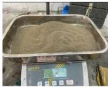
Fig.24: Sol sec concassé.
