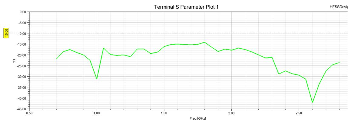
**FIGURE 3.16-LES COEFFICIENTS DE TRANSMISSIONS S12 ET S21.**
