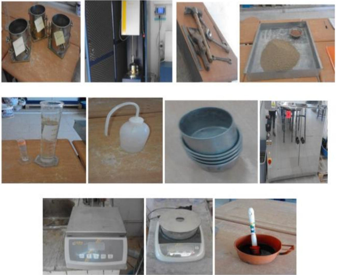
Figure III.9 : Appareillage – essai Proctor.
