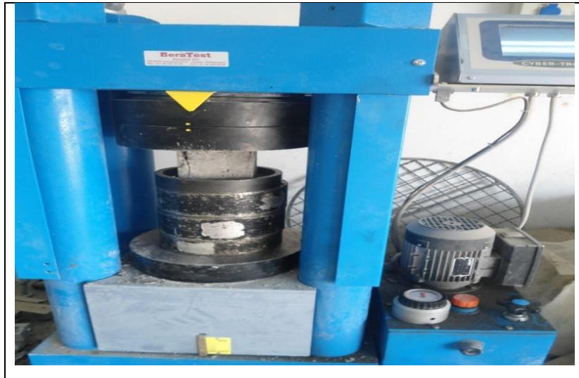
Photo III.14: Presse hydraulique de compression.
