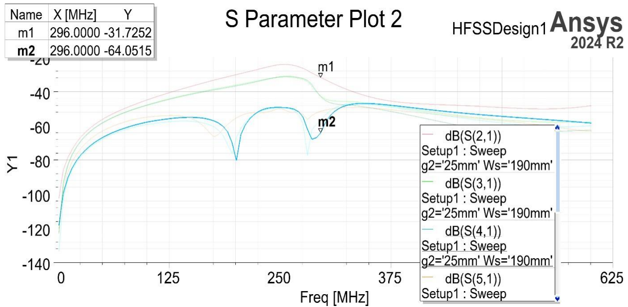
Figure 3.12: The simulated transmission parameters S_{il} of the loaded 8 channel MTL
