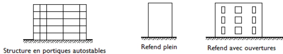
Figure II.10 : Exemples de contreventements plans.
