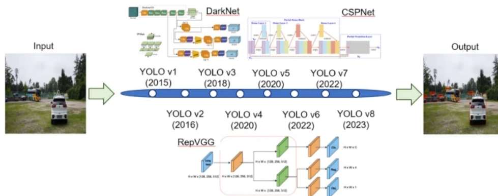
Figure 2.4: YOLO Evolution Timeline: Architectural Backbones and Version Progression (2015–2023)
