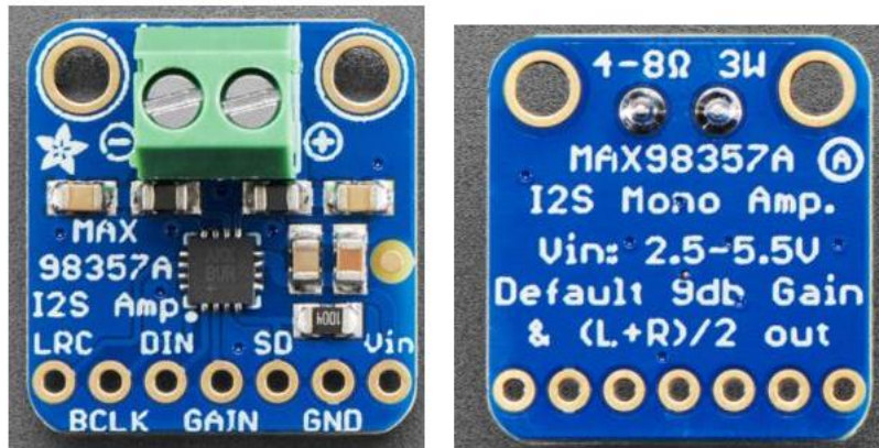
Figure 2. 17— Audio Amplifier MAX98357A (I2S)
