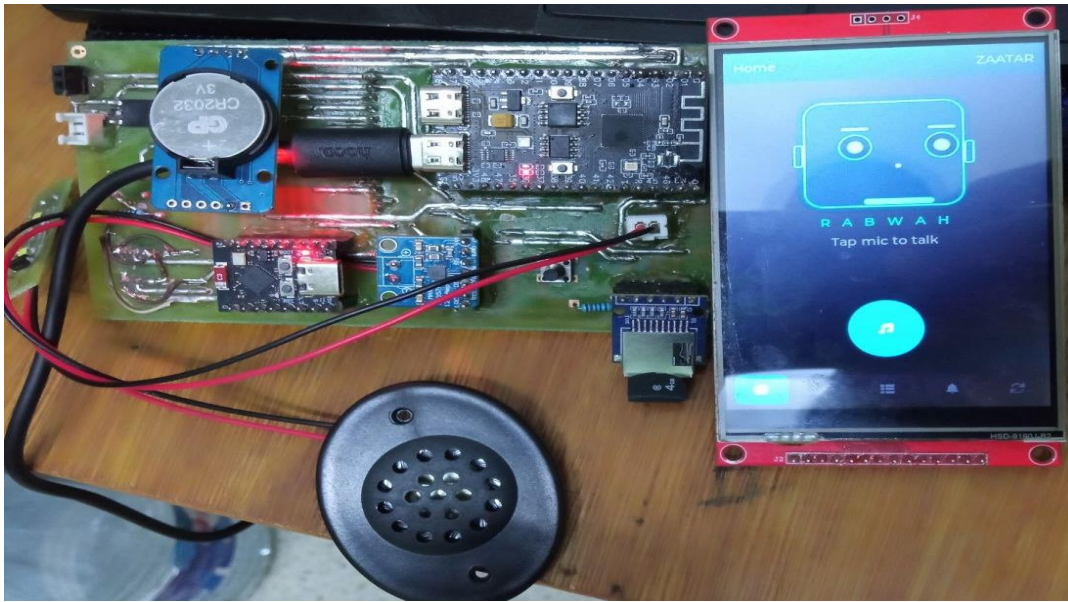
Figure 3. 1— Prototype test bench: custom PCB with all integrated subsystems, Home screen active
