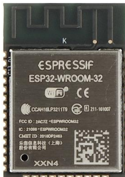
Figure II.4. ESP 32 wroom 32 WI-FI + BLuetooth Antenna [22].
