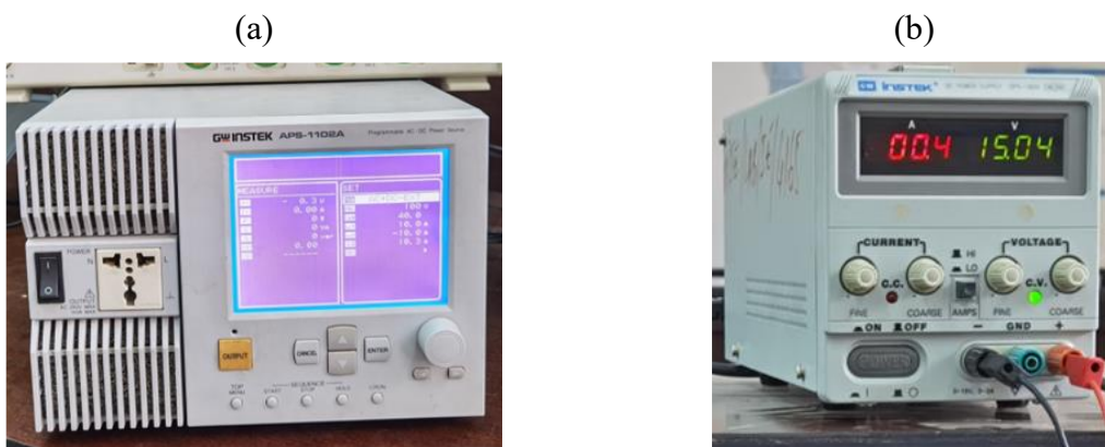
Figure III.2. (a) Programmable power supply and (b) DC power supply.
