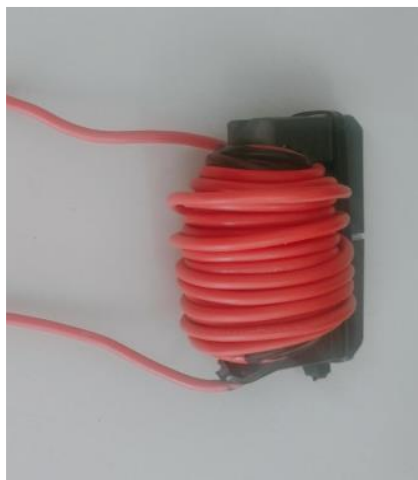
Figure III-8 Inductor component (0.70 mH)
