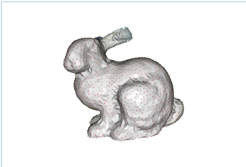
Figure 2. 6: Generated Rabbit Mesh Using BP
