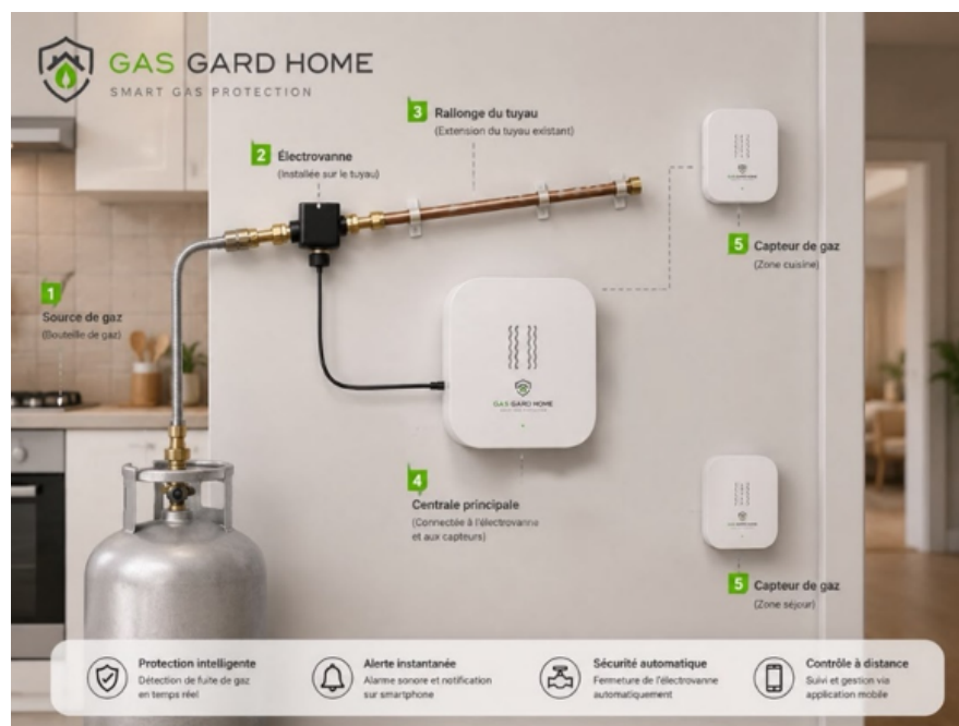
FIGURE 3.5 – Prototype final du système GAS GUARD HOME
