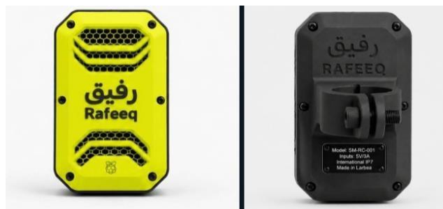
Figure 3.5. Assembled scooter IoT enclosure containing the Raspberry Pi 3B+, the SIM800L modem, the GPS receiver, and the buck converters, prior to mounting on the scooter chassis.
