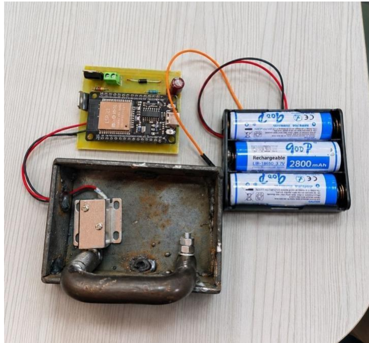
Figure 3.7. Complete locking subsystem of the Rafeeq docking station, showing the electronic control board (top), the 12 V electromechanical Solenoid that drives the steel pin housed inside the station body (bottom-left), and the captive steel ring permanently attached to the scooter frame that the pin captures when the scooter is docked (bottom-right).
