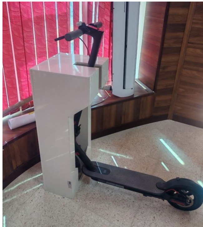
Figure 3.9. Assembled prototype of the Rafeeq docking station with a scooter docked into the slot. The mechanical capture is implemented by the captive ring permanently attached to the scooter frame, which engages the Solenoid pin housed in the station body.
