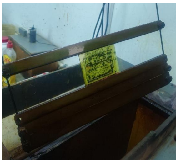
(a) Board in the ferric chloride bath
