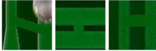
Figure 1.3: An example of the Short defect.
