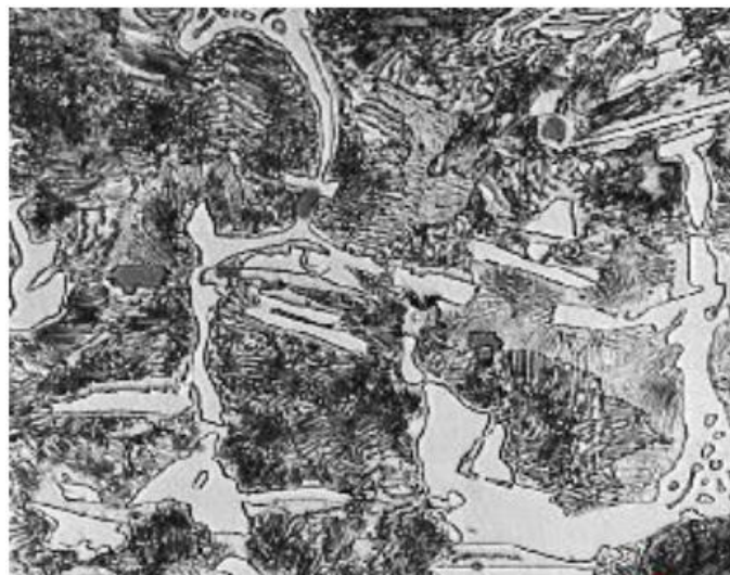
Figure 3.6 White cast iron structure
