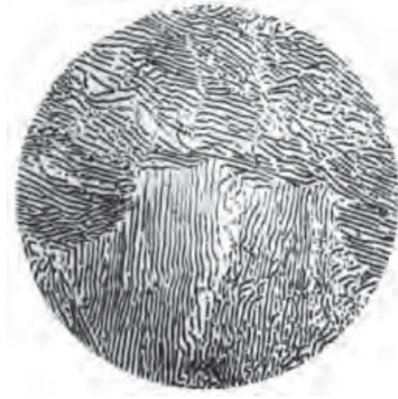
Figure 2.4 Microstructure showing lamellar nature of pearlite ( \times 1200 ).
