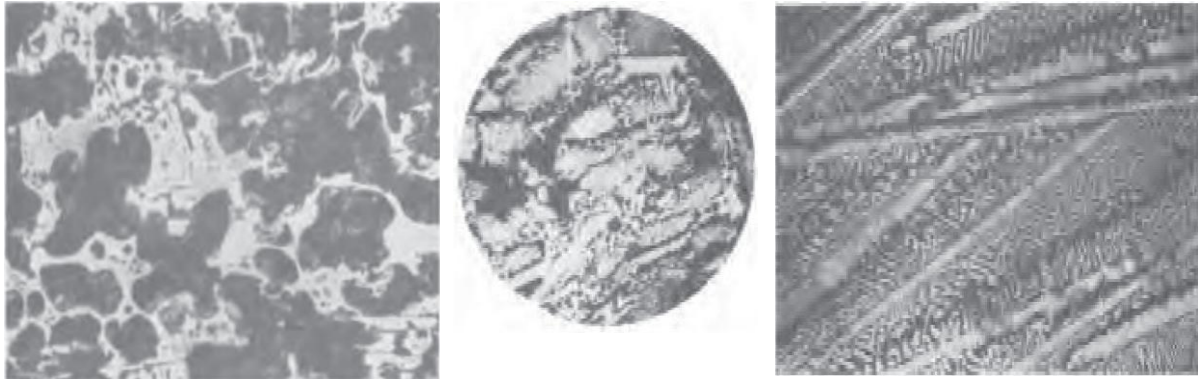
(a) Hypoeutectic cast iron (ledeburite + pearlite + cementite), \times 200
