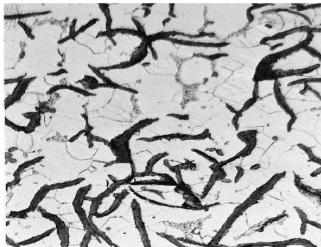
Figure 3.4 Gray cast iron structure
