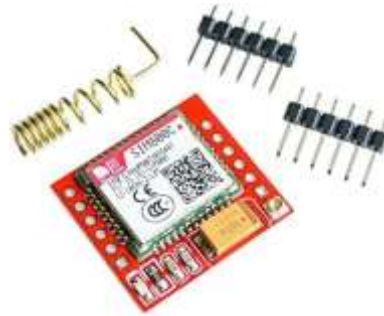
Figure III-7 Module de communication (GSM SIM800L).
