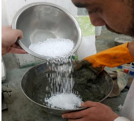
Figure 25: Incorporation du polystyrène expansé (EPS)
