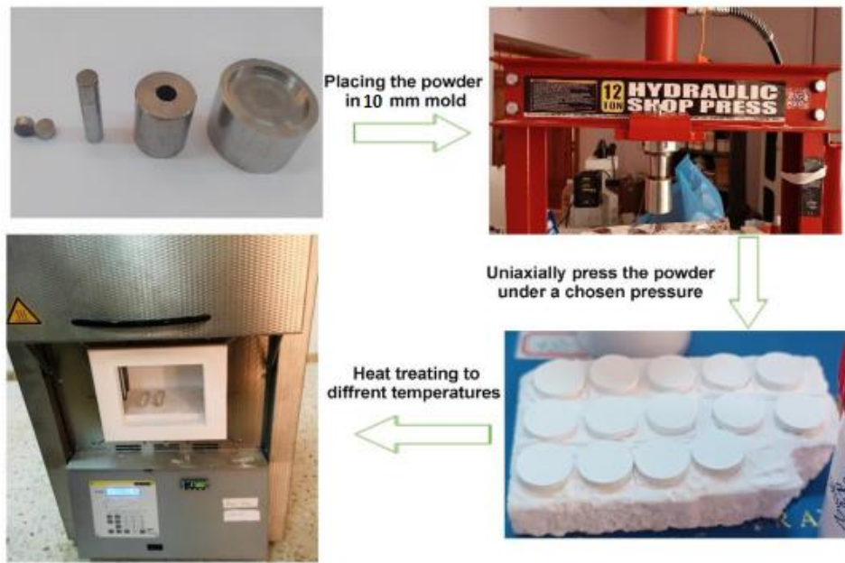
Figure II.3: The process of molding and sintering samples.
