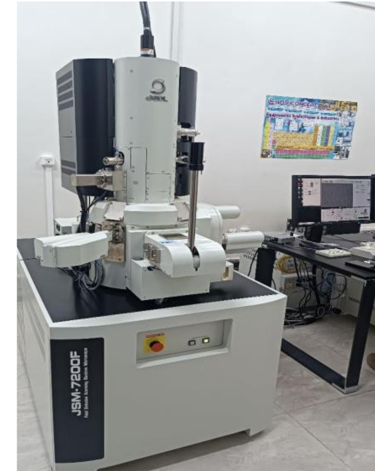
Figure II.11: Scanning electron microscopy (SEM) combined with Energy Dispersive Spectroscopy (EDS) (univ of Bejaia).
