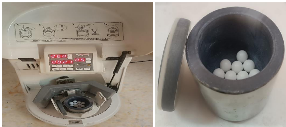
Figure II.2: Planetary ball mill (Fritsch P6) and zirconia balls
