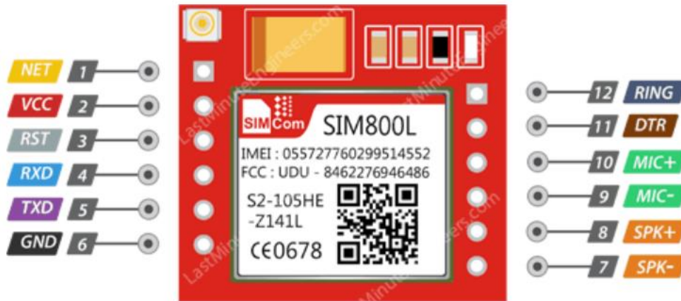
Figure 25 : GSM SIM800L Pinout [14].
