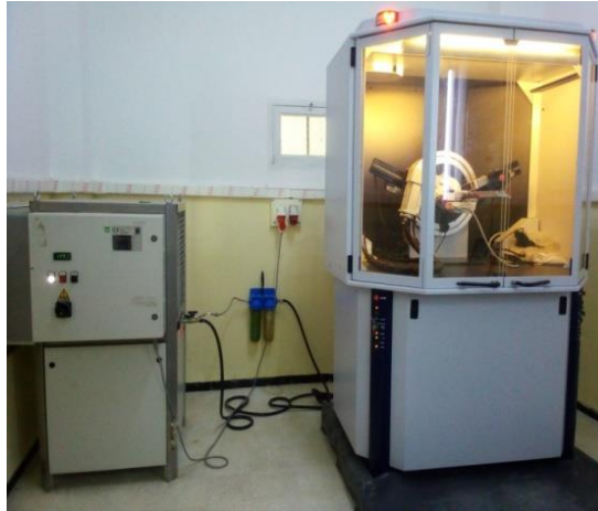
Figure II.21: Photo de diffraction des rayons X (DRX) de type BRUKER D8.
