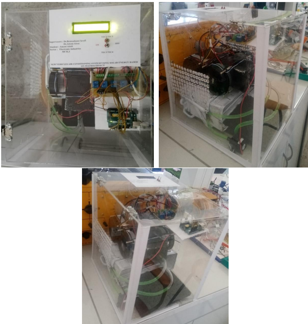
Figure II.13 : Realization of vehicles air conditioning system finished product.
