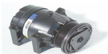
Figure I.1.5 : A typical air conditioning compressor.
