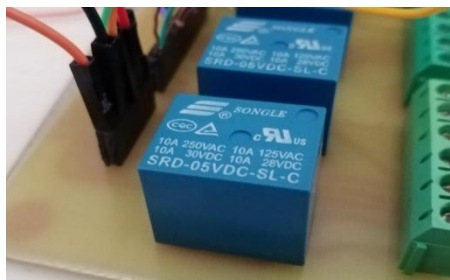
Figure II.3 : SRD 5V Relay.
