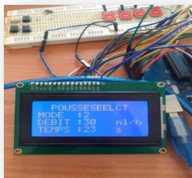
Figure III.11: injection en cours mode 2
