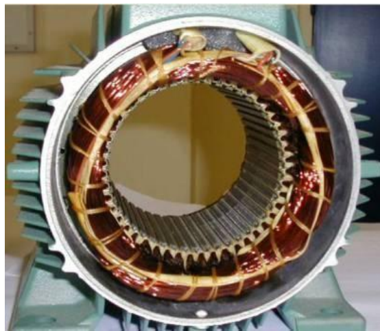
Figure (I.2) : Stator de la machine asynchrone
