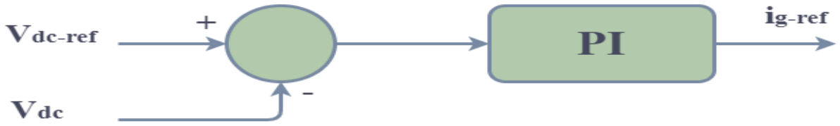
Figure II.12: PI DC-link voltage controller.
