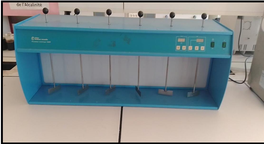
Figure I-6 : Jar-test.
