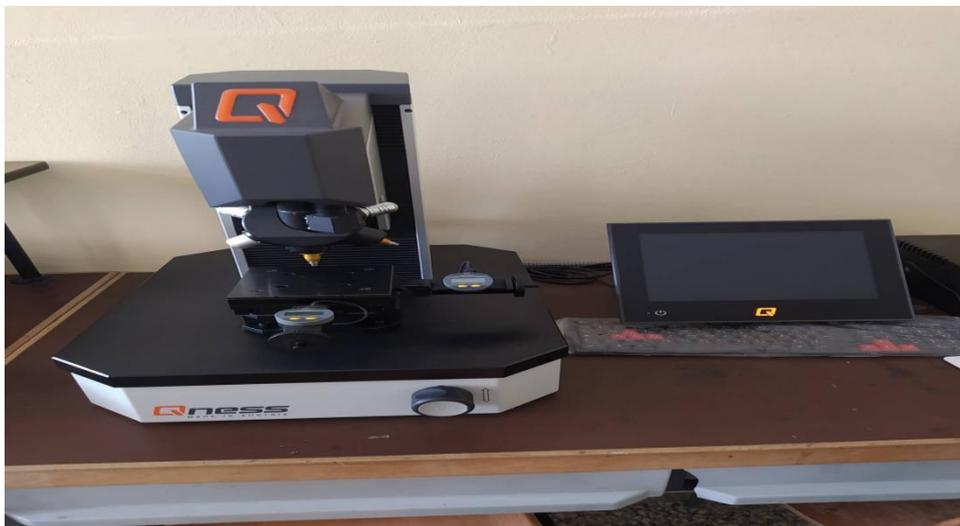
Fig 3.5 Machine d'indentation Qness 30
