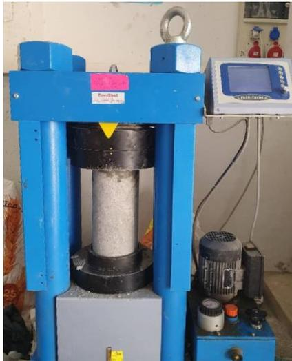
**Figure 3. 6:** Machine de compression.
