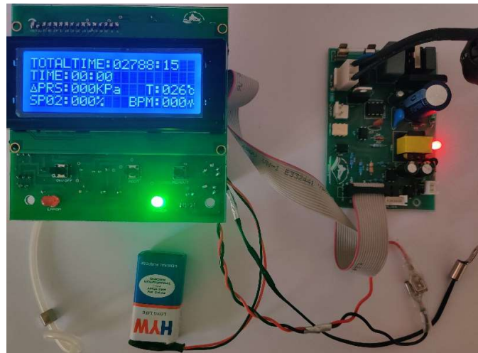
Figure 3.34: Practical realization of power supply and display and control boards.
